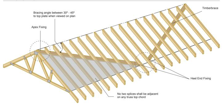
Top chord bracing may be affected by using (minimum) 75 x 38mm (F8) hardwood or 70 x 35mm (F5) softwood.
